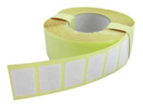
The ever-popular MIFARE Classic 1K chip from NXP in sticky label format. Operates at 13.56 MHz wireless frequency, according to the ISO 14443A standard, and contains 1Kbytes of read/write memory that can be used for multiple applications.
